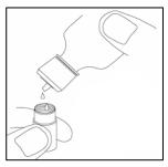
4. Fill a new membrane cap with the appropriate electrolyte solution that has been prepared according to the directions on the bottle. Polarographic sensors use electrolyte that is in a white labeled bottle (KCl/Na<sub>2</sub>SO<sub>4</sub>). Galvanic sensors use electrolyte that is in a blue labeled bottle (NaCl). Be very careful not to touch the membrane surface during this process. Lightly tap the side of the membrane cap to release air bubbles that may be trapped.
